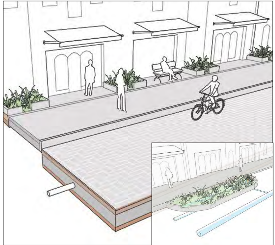
Figure 34. Bioswale Stormwater Design
